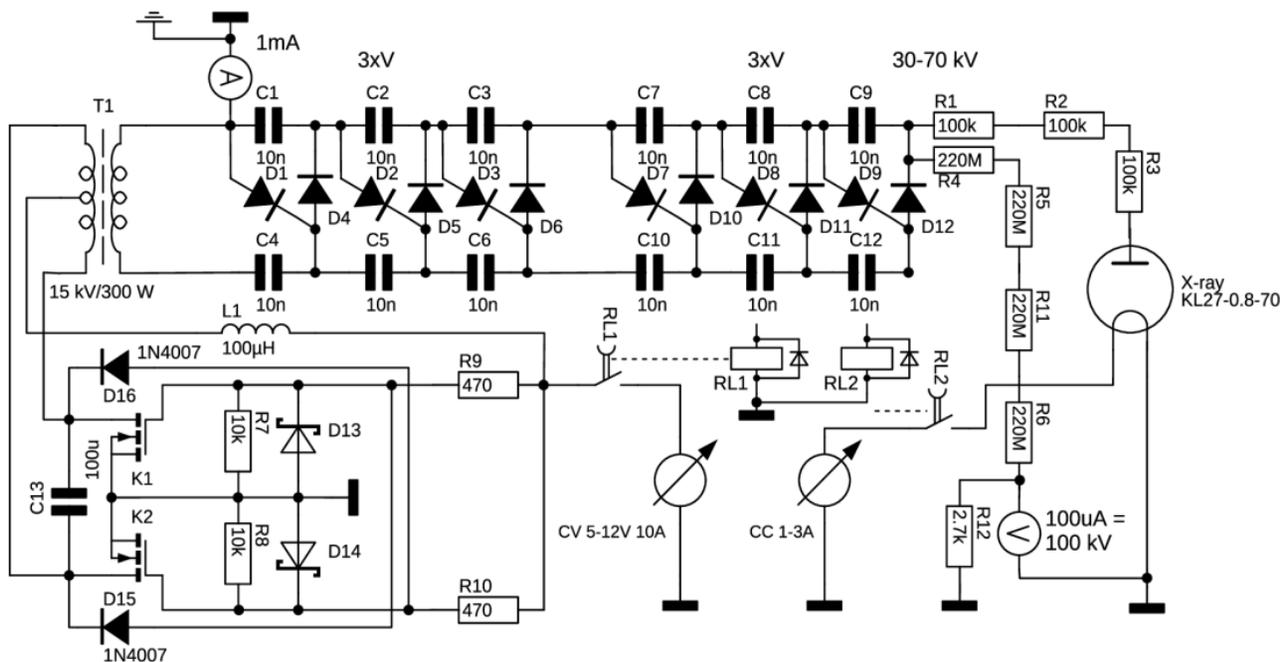
Fig. 3. Electronic schematic of the low-cost X-ray source
