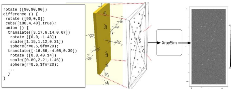
Fig. 6. Modelling of a die casted aluminum plate with gas pores using Monte Carlo simulation. Geometric parameters of real measure pores are used to create synthetic pores at random positions. (Left) Programmatic CSG model (Center) Rendered 3D model with synthetic pores / holes (Right) Simulated X-ray Image
