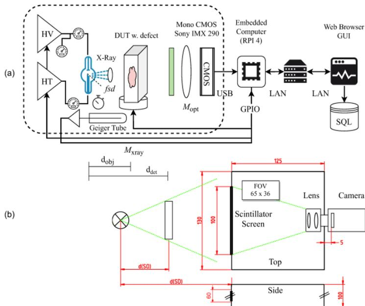
Fig. 1. Low-cost X-ray Radiography and CT instrument (a) General overview (b) Details of the detector (all dimensions in mm)
