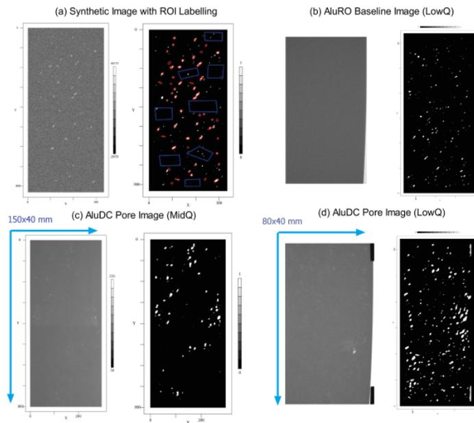
Fig. 8. Feature marking for different X-ray images using two measuring instruments and synthetic images. Low-Q images have a different scaling and region compared to the Mid-Q and synthetic X-ray images. aluDC: Die casted aluminum plate with pores, aluRO: Rolled and polished aluminum plate without pores.
