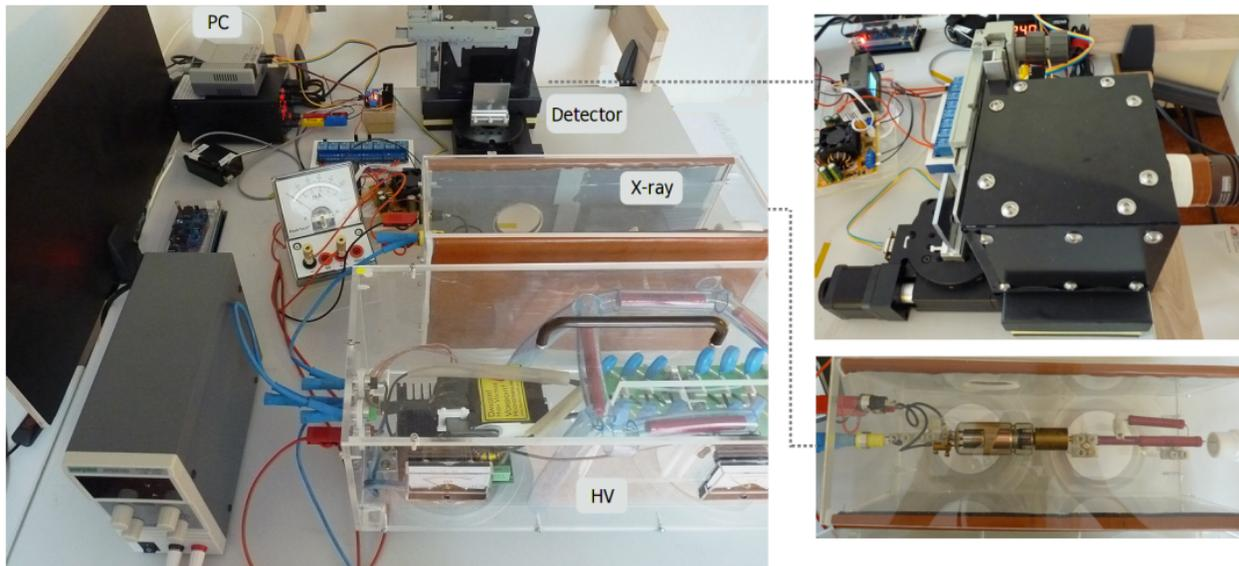
Fig. 2. Prototype of the low-cost X-ray Radiography and CT instrument
