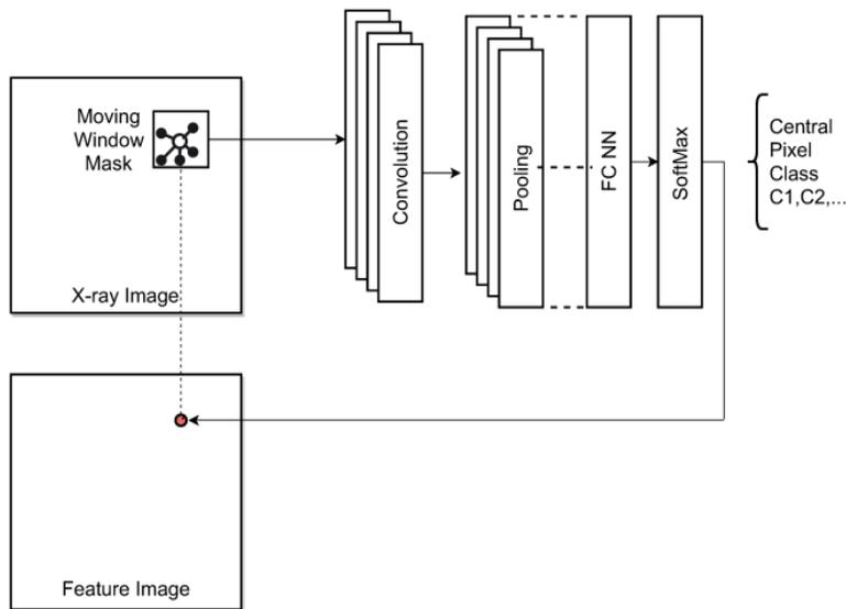
Fig. 7. Semantic pixel classifier applied to X-ray single projection images to detect and mark hidden defects
